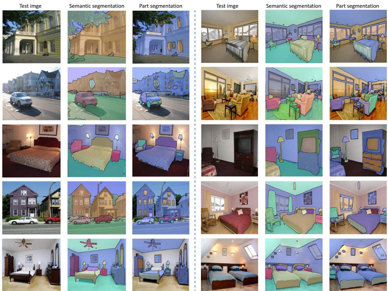
Fig. 17 Object and part joint segmentation results predicted by UPerNet (Xiao et al. 2018). Object parts are segmented based on the top of the corresponding object segmentation mask
